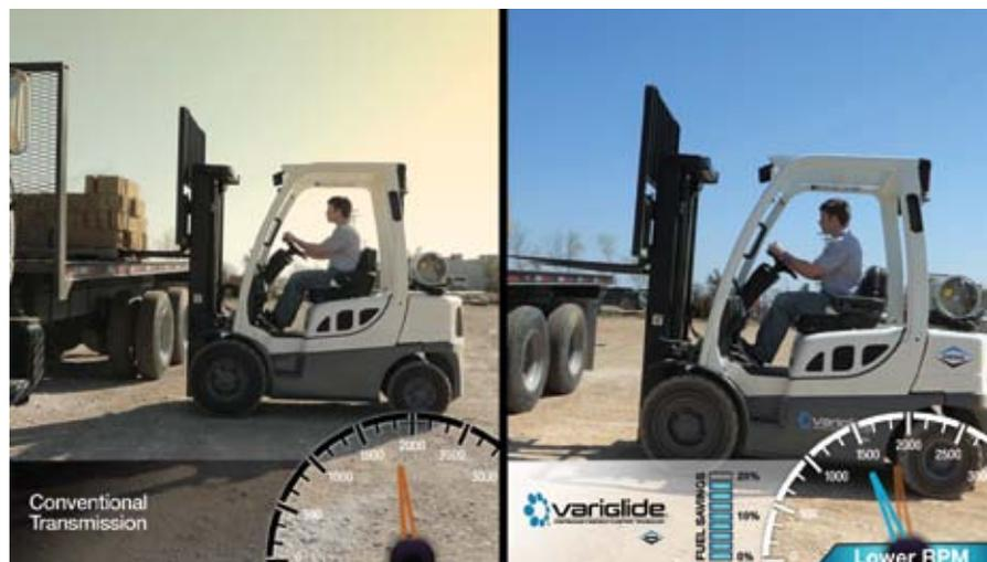
VariGlide™ transmission technology reduces engine stress, reduces fuel consumption, and increases productivity.
